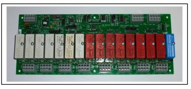
of drive and receive circuit options. G4 and G5 modules also may be used. SM and M type modules may also be inserted to the standard footprint connections, but do not provide screw-down security. Any of these modules may provide UL, CSA, and/or CE approved interfaces to external circuitry as required (refer to specific module data). The sixteen lines are jumper-configurable for input or output signaling to match the installed module type.
